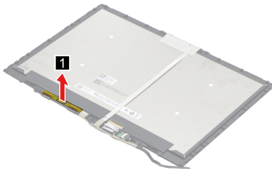
Figure 23. Peel off the tape
