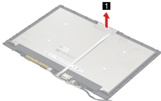
Figure 25. Remove the camera foil
