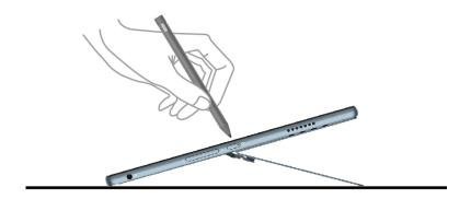
The kickstand is multi-positional. You can adjust the kickstand to various angles for a comfortable user experience. Do not pick up the computer when the kickstand is open. Otherwise, the computer might overheat, and could cause discomfort or even a skin burn to you.
