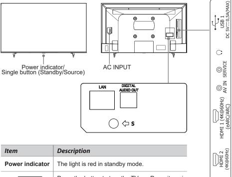
Press the button to turn the TV on. Press it again<br/>to bring up the control menu and move the focus<br/>between different inputs. Long press the button<br/>to make a selection.
