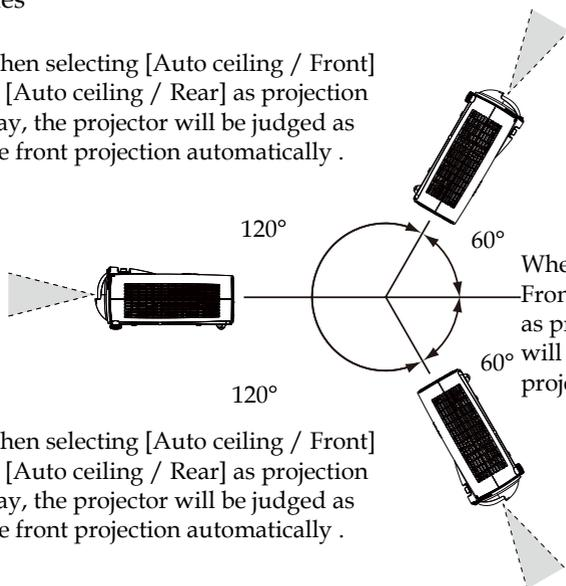
When selecting [Auto ceiling / Front] or [Auto ceiling / Rear] as projection way, the projector will be judged as the ceiling projection automatically .
