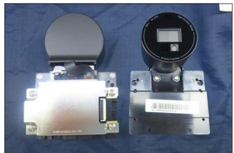
Tear off 1pcs aluminum foil for uncovering the fan, then use a Philips-head screwdriver to remove 3pcs screws for unlocking the fan with the unit.
