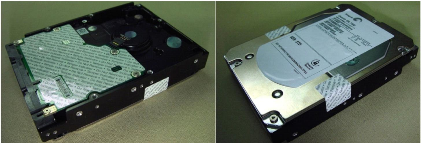
**Figure 6. Example of FIPS tamper evidence labels.**
