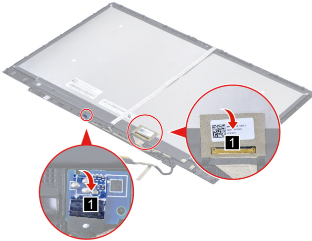
Figure 22. Peel off the two pieces of tape
