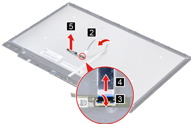
Figure 21. Remove the camera board
