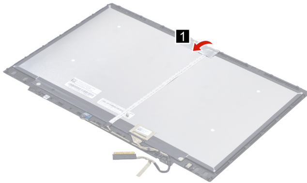
Figure 20. Peel off the camera AL foil
