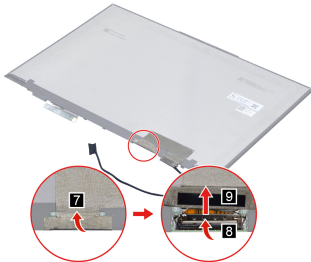
Figure 30. Remove the EDP cable
