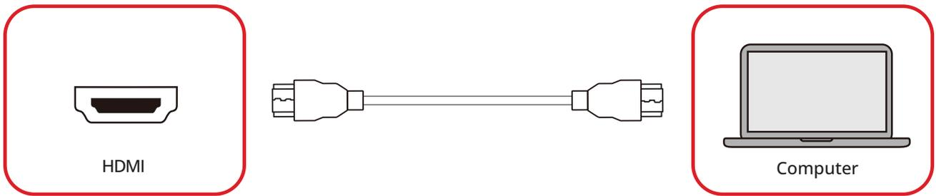
Connect an HDMI cable from your external device to the **HDMI 1/HDMI 2/HDMI 3/HDMI 4** port on the display.
