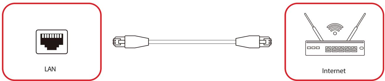
To connect to a network, connect an Ethernet cable to your network, then connect the other end to the **LAN** port of the display.
