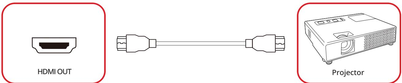
To output video via an external display device, connect an HDMI cable to the **HDMI IN** port of your external display device, and the other end to the **HDMI OUT** port of the display.
