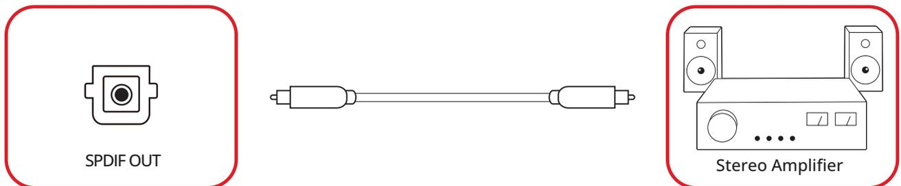
**NOTE:** The **SPDIF Out** port is accessed by removing the System Control Box Cover.
