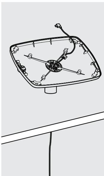
**4** Feed the tablet cable through the Bouncepad Case & Flex.
