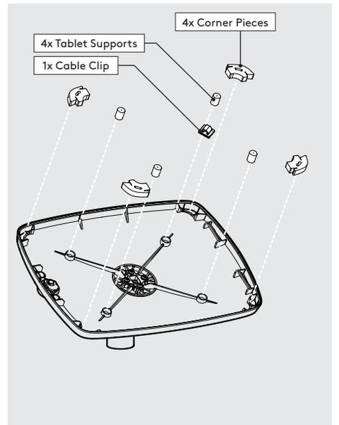
**3** Install the Tablet Setup Kit. Each kit is specific per tablet device and Bouncepad Case.
