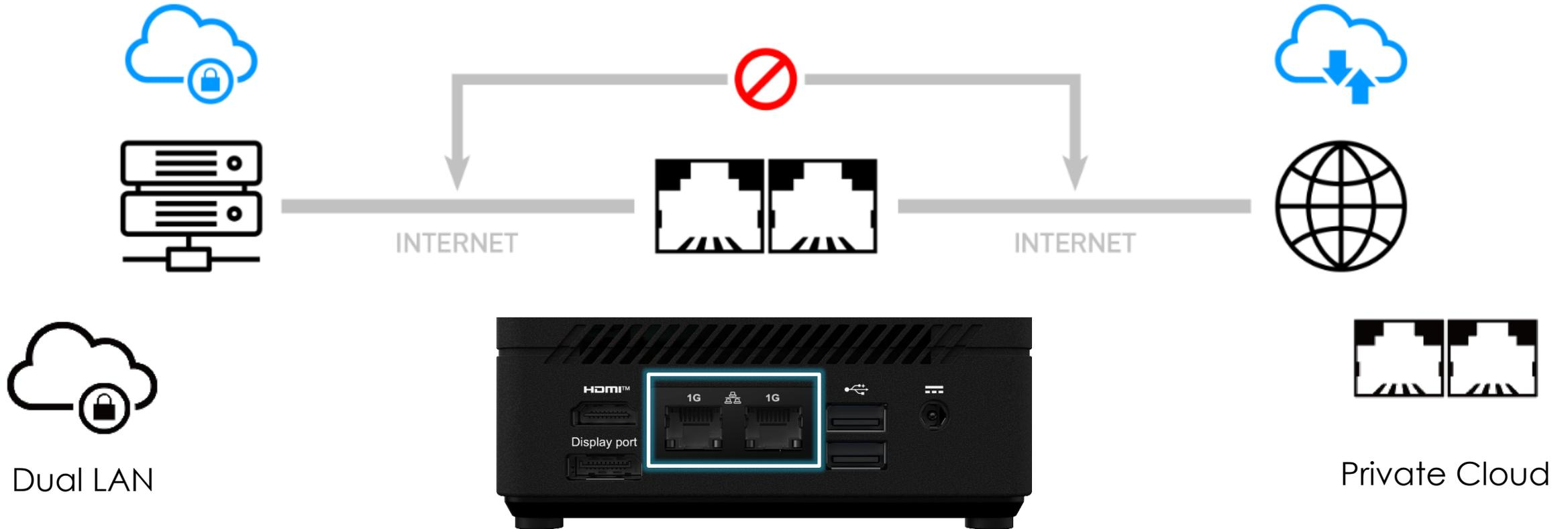
If one of the LAN ports fails, you can still access the network using the other port. Utilizing two LAN ports provides redundancy to the network connection, significantly enhancing data transfer reliability and availability.
