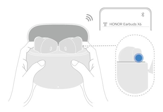
Restore factory settings: Rest the earbuds in the case, keep the lid open, press the touch control areas of both earbuds for 10 seconds simultaneously. Red light blinking indicates the earbuds are restored to factory settings and the earbuds re-enter the pairing mode. While wearing both earbuds, press the touch control areas of both earbuds for 12 seconds simultaneously to restore factory settings.
