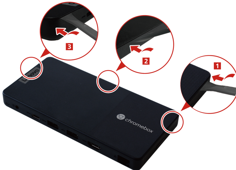
Figure 5. Pry up the latches
