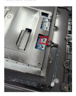
Tear off "MYLAR USB board" from "Main Shielding"
