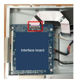
Insert "USB B board to Interface board wire" to "USB B board" and assemble "USB B board" to "Main Shielding"
