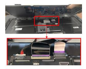
S21 Lock 4 screws to fix "Main Shielding" on "Panel"
