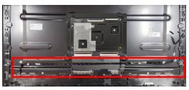
S20 Disassemble "Middle Frame" from "ASSY CHIN" and "Panel"
