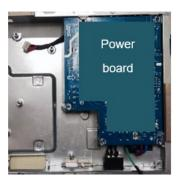
Unplug "Power board to DC-DC Board wire" from "Power board"
