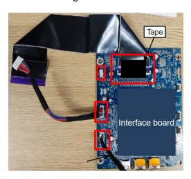
Insert "Interface board to Panel FFC (51P)" to "Interface board"
