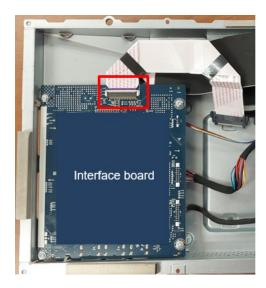
S29 Disassemble "DC-DC board" from "Main Shielding"
