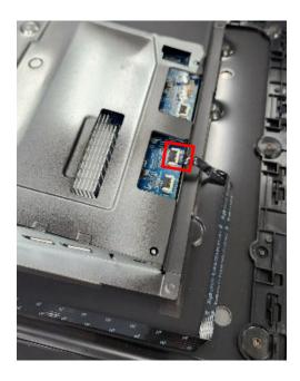
S23 Attach a "GASKET" to "USB board"
