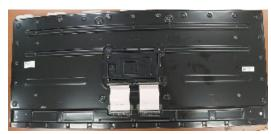
S24 Tear off "LENS Board FFC" from "Middle Frame"
