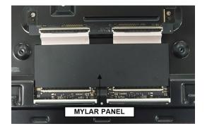
Assemble a white "MYLAR PANEL" to "Panel"
