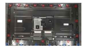
(Screw Torque-MF: 4-4.5 kgf) (Screw Torque-CHIN: 1.5-2.5 kgf) Tear off "LENS board FFC" from "Panel"
