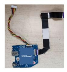
Assemble "USB board" to "Middle Frame" and lock a screw to fix it
