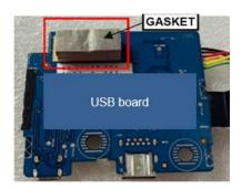
Insert below cables to "USB board" a. USB board to USB B board wire b. USB board to USB B board FFC
