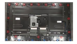
(Screw Torque-MF: 4-4.5 kgf) (Screw Torque-CHIN: 1.5-2.5 kgf)
