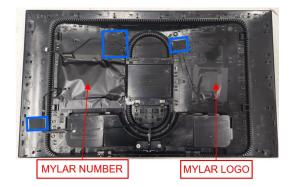
Unlock 4 screws to disassemble "ASSY LED MOUDLE" from "Rear Cover"
