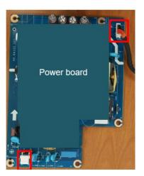
Assemble "Power board" to "Main Shielding"
