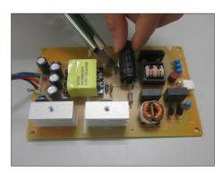
S17-4 Take out bulk cap. pin solder with soldering iron and absorber.
