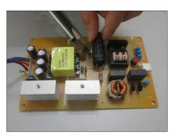
S17-2 Ensure cutting path within the glue, don't touch bulk cap. or PCB.
