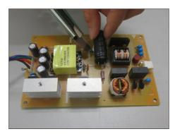
S17-3 Cut into the bottom of bulk cap. and pullit up carefully.
