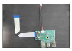
Use a Philips-head screwdriver to remove 1pcs screw for unlocking the joystick board with middle frame, then release the key cable by tearing off 2pcs tapes, then release the joystick board from the hooks of the middle frame.
