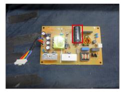
S17-1 Cut the glue between bulk cap. and PCB with a knife.
