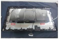
Put the middle frame into a fixture jip, then tear off the mylar tape, and then use a Philips-head screwdriver to remove 1pcs screw for unlocking the power key board with the middle bezel.
