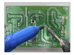
S17-5 Lift the bulk cap. up and away from the PCB.
