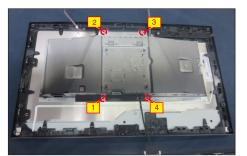
Tear off 2pcs tapes on the back of the power key cable, then lift up the middle bezel and remove the middle bezel.
