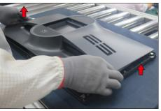
Remove the rear cover, then tear off 1pcs aluminum foil for uncovering the EDP connector, then disconnect power key cable and joystick key cable away from the connectors of the board. Tear off 1pcs shading mylar, then disconnect the panel lamp connector, then release the cable from the hooks of the middle frame and bracket.
