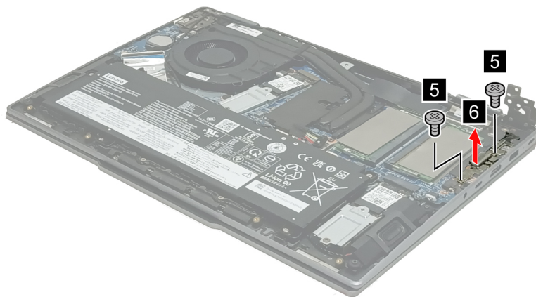
Figure 22. Remove the I/O bracket
