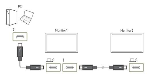
Dual display (daisy chain) support depends on your PC and the connected Thunderbolt™ 3 / 4 cable. The Thunderbolt™ 4 port on your PC must support dual 4 K @ 60 Hz output, and the particular 40Gbps Thunderbolt™ 3 / 4 cable need to be purchased separately. For detailed specification of the Thunderbolt™ 3 / 4 cable, visit the official Thunderbolt website.
