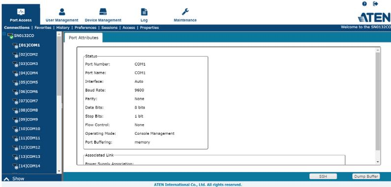
From here you can use the **Telnet**, **SSH**, and **Dump Buffer** buttons at the bottom of the page.
