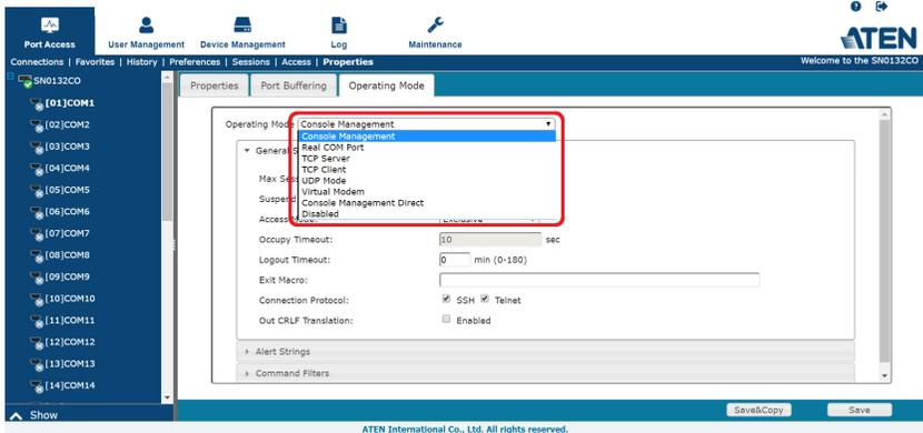
The **Operating Mode** is selectable from the *Port Access - Properties* page, under the *Operation Mode* tab, as shown above. From this page you can set the Port Operating Modes that are discussed in this chapter. See *Operating Mode*, page 73, for further details on configuring all the settings.
