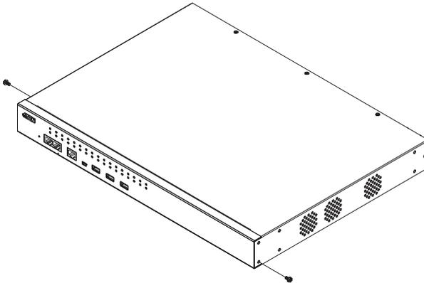
2. Use the M3 x 8 Phillips head hex screws supplied with the rack mount kit to screw the rack mounting brackets into the front of the unit.
