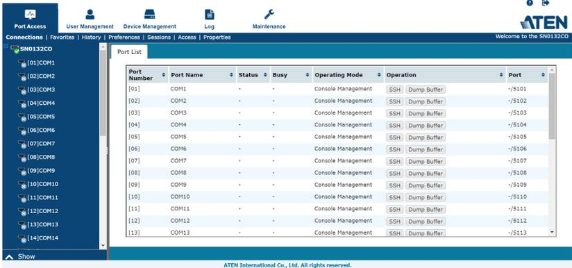
The *Connections* page is organized into several main areas. All the devices, ports, and outlets that a user is permitted to access are listed in the Sidebar at the left of the page.
