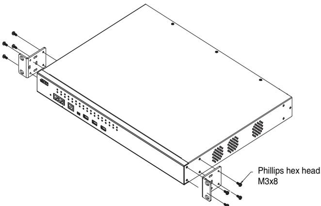
3. Position the device in the front of the rack and align the holes in the mounting brackets with the holes in the rack.
