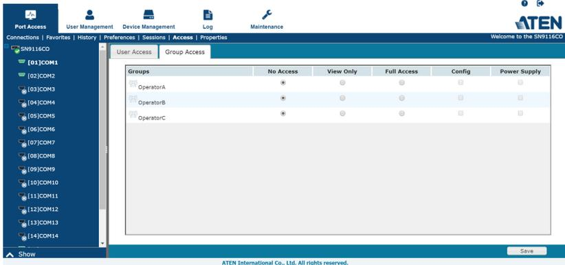
Use the radio buttons to configure access rights on the *User Access* and *Group Access* page. The meaning of the columns are given in the table, below:
