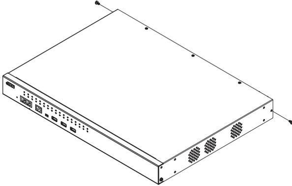
2. Use the M3 x 8 Phillips head hex screws supplied with the rack mounting kit to screw the rack mounting brackets into the rear of the unit.
