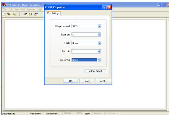
Bits per Second: **9600**, Data Bits: **8**, Parity: **None**, Stop bits: **1**, Flow Control: **None**.
