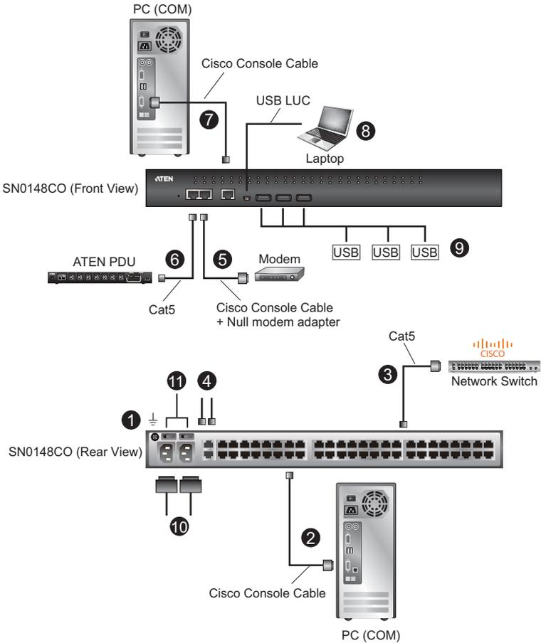
**Note:** The example above shows a SN0148CO Serial Console Server. The SN0108CO / SN0116CO / SN0132CO units have the same ports and switches but with slightly different layouts. See *Components*, page 9 for details.
