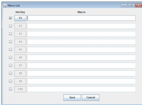
Simply check a box, type in the text macro and click **Save**. Use the associated function key (F1-F12) to run the custom text macro(s) you created. Terminal Application
