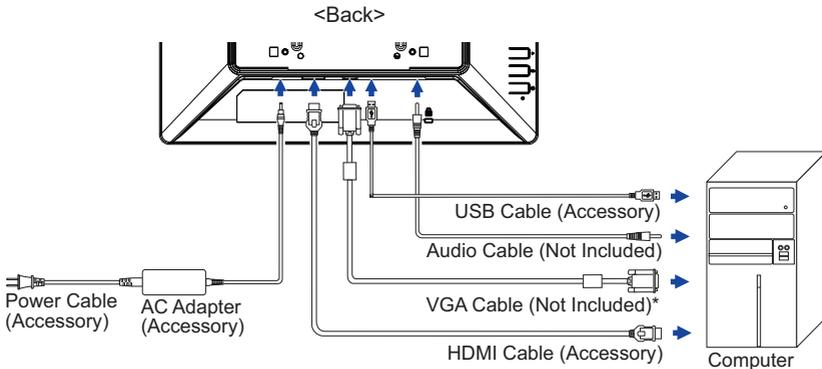
\* VGA cable is not supplied with the monitor. If you use low quality VGA cable, it may cause a result of electro-magnetic interference. Please contact the iiyama Support Centre in your country if you wish to connect the monitor via the VGA input.
