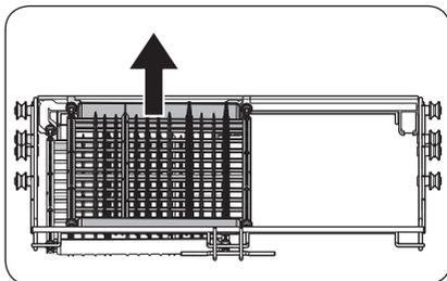
3. Make sure that the tray shaft is positioned at the opening hole. Then, pull up the tray to remove.
