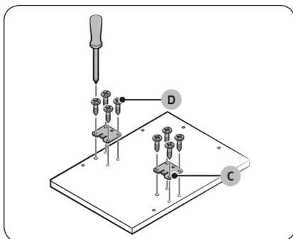
4. Tighten the door bracket (C) with 8 screws (D, Ø4 X 14) as shown in the figure.
