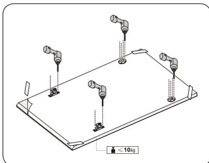
1. Place the installation template on the back of the custom panel and fix it temporarily using transparent tape. Note that the rear of the custom panel will be attached to the dishwasher door.
