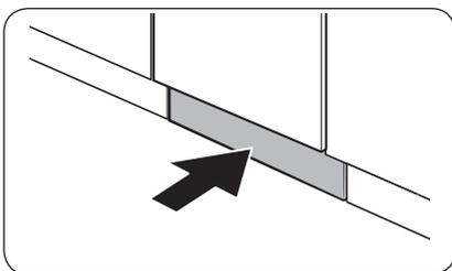
3. Push the skirting board with the brackets into the bottom of the dishwasher as shown.
