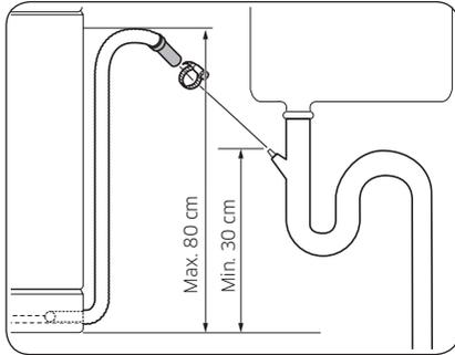
1. Connect the drain hose to the drain outlet.
