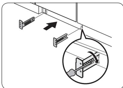
3. Push the kick plate with the brackets into the bottom of the dishwasher as shown.
