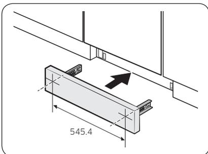
2. Insert the pre-cut skirting board into the brackets first, and then tighten the screws to fix the board. See the figure on the left and make sure the brackets are positioned in the correct place.
