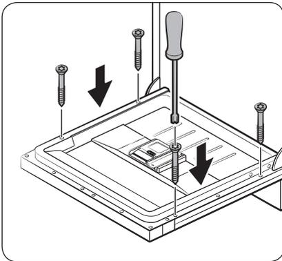
10. Secure the custom panel to the door by fastening the 4 screws (Ø3.5 X 45).
