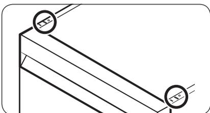
1. Insert the provided brackets into the top front holes of the dishwasher as shown.
