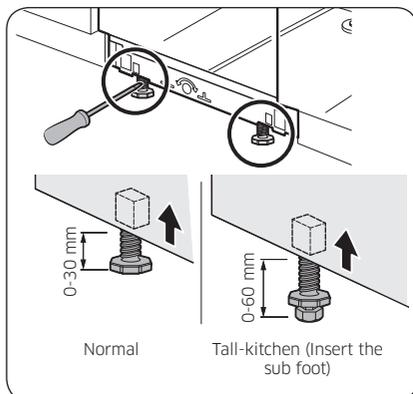
You can adjust the height of the dishwasher to level it. Note that in these steps, the dishwasher is currently inserted halfway.
