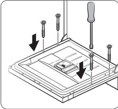
13. Secure the custom panel to the door by fastening the 4 screws ( $\text{Ø}4 \times 43$ ).
