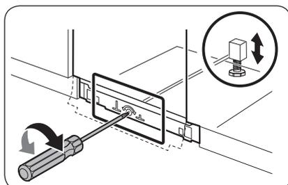
3. To adjust the rear height, insert a cross head(+) screwdriver in the bottom centre of the dishwasher.
