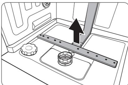
1. Open the door, and then pull out the lower rack. The lower nozzle is visible on the bottom.
