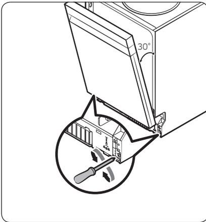
14. Adjust the spring level while the door is approximately opened at 30 degrees. The door should hold its position, and should not fall open.
