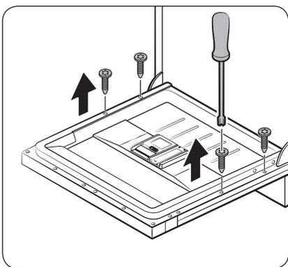
12. Open the dishwasher door and remove the 4 screws.
