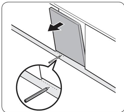
1. Put the skirting board on the bottom of the dishwasher.
