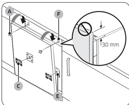
5. Insert the door brackets (C) on the custom panel to the holes (E) on the dishwasher door to fix the custom panel.
