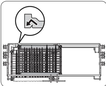
2. Gently lift the left shaft of the tray and move up to the opening hole of the chassis.
