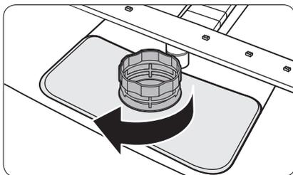
4. Remove any dirt and impurities from the micro filter and the Coarse filter.
