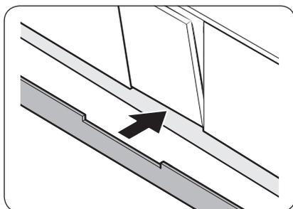
4. Attach the cut skirting board to the bottom of the dishwasher. Make sure the board does not interfere with the door of the dishwasher.
