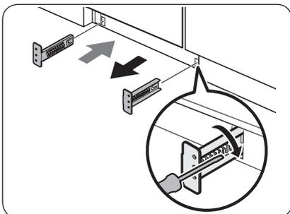
1. Insert the provided brackets to the bottom of the dishwasher. Turn them into position.
