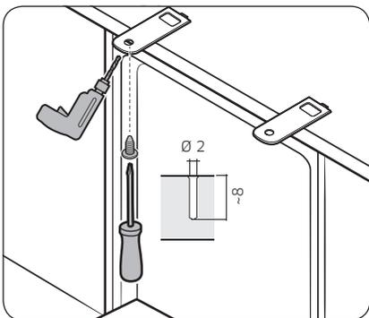
3. Tighten the 2 screws ( $\varnothing 4 \times 14$ ) to fix the brackets.
