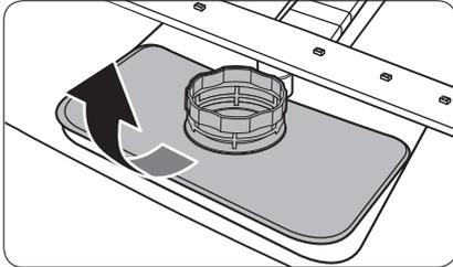
3. Remove the Coarse filter, and then the cylindrical micro filter underneath.
