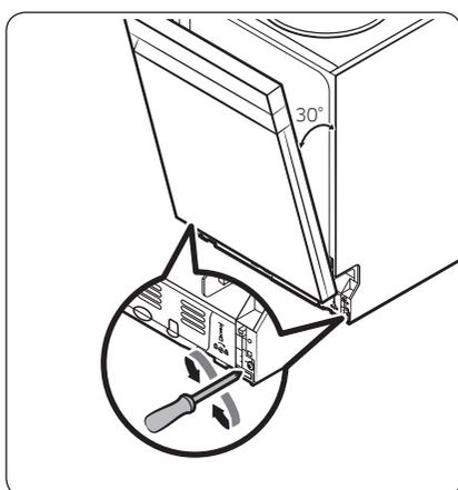
8. Adjust the spring level while the door is approximately opened at 30 degrees. The door should hold its position, and should not fall open.
