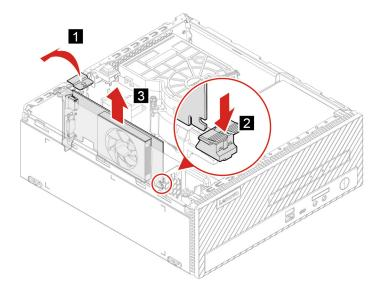
**Note:** If the card is held in place by retaining latch, press the latch as shown to disengage the latch. Then, gently remove the card from the slot.
