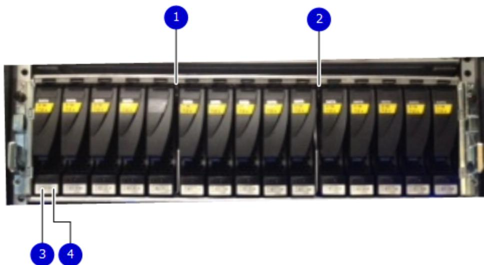
Figura 181. LEDs do painel frontal
