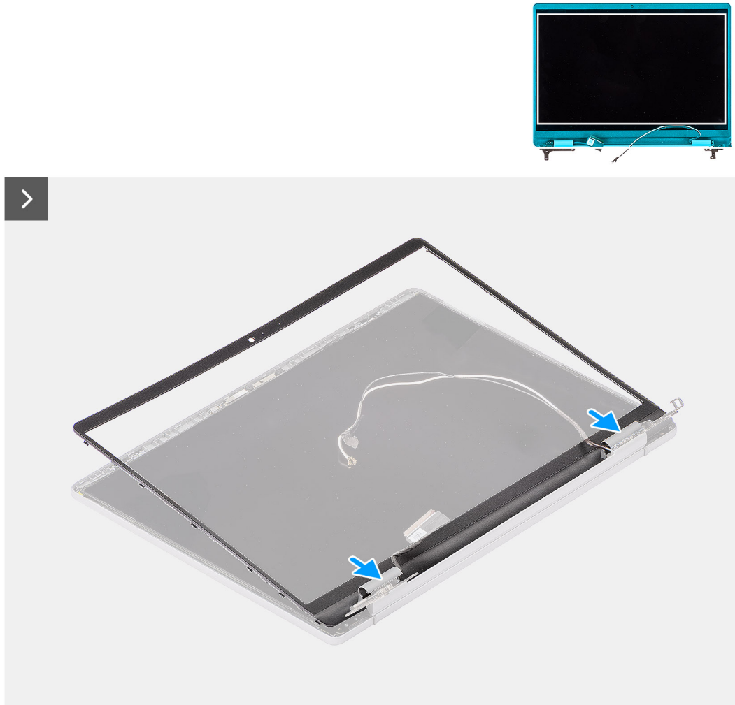
Figure 51. Installing the display bezel
