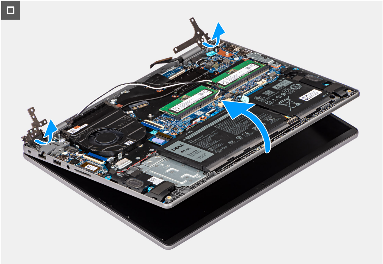
Figure 43. Removing the display assembly
