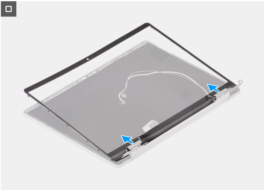
Figure 49. Removing the display bezel
