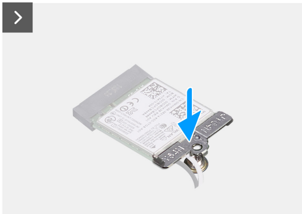
Figure 19. Installing the wireless card
