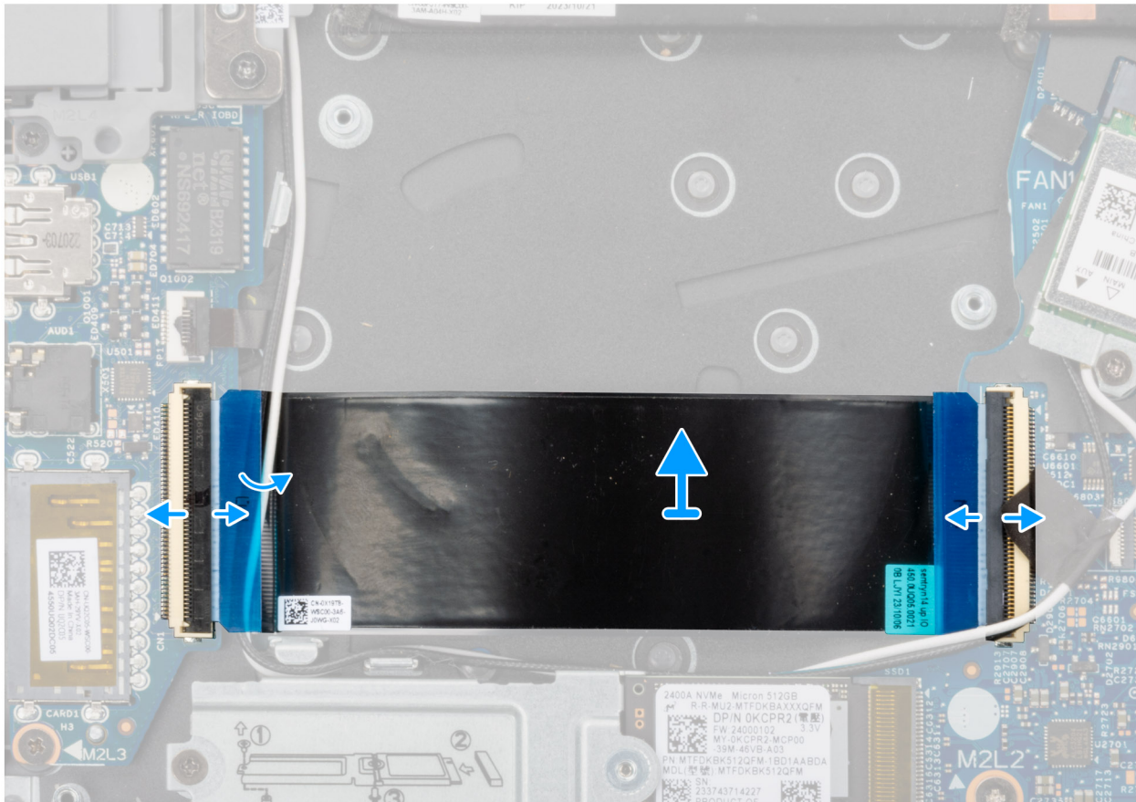
Figure 34. Removing the I/O-board cable
