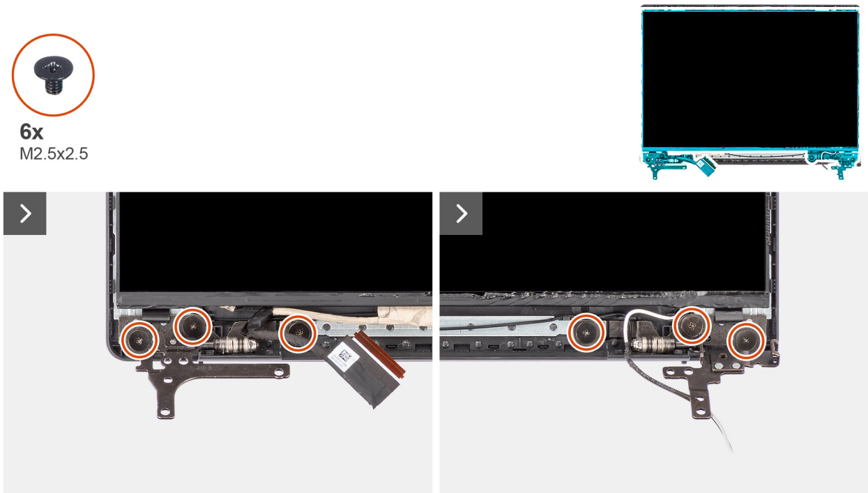
Figure 53. Removing the display panel
