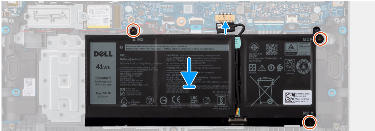
Figure 23. Installing the battery
