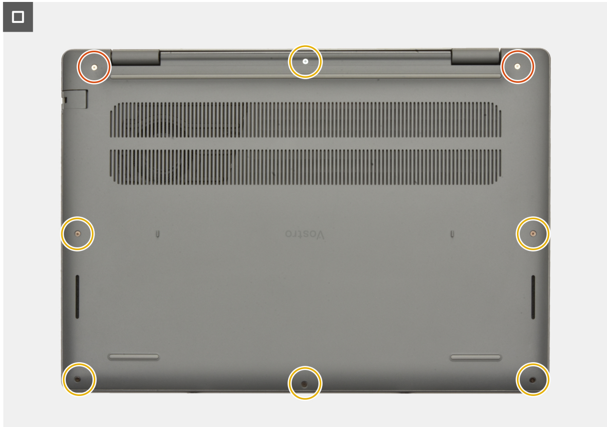
Figure 13. Installing the base cover
