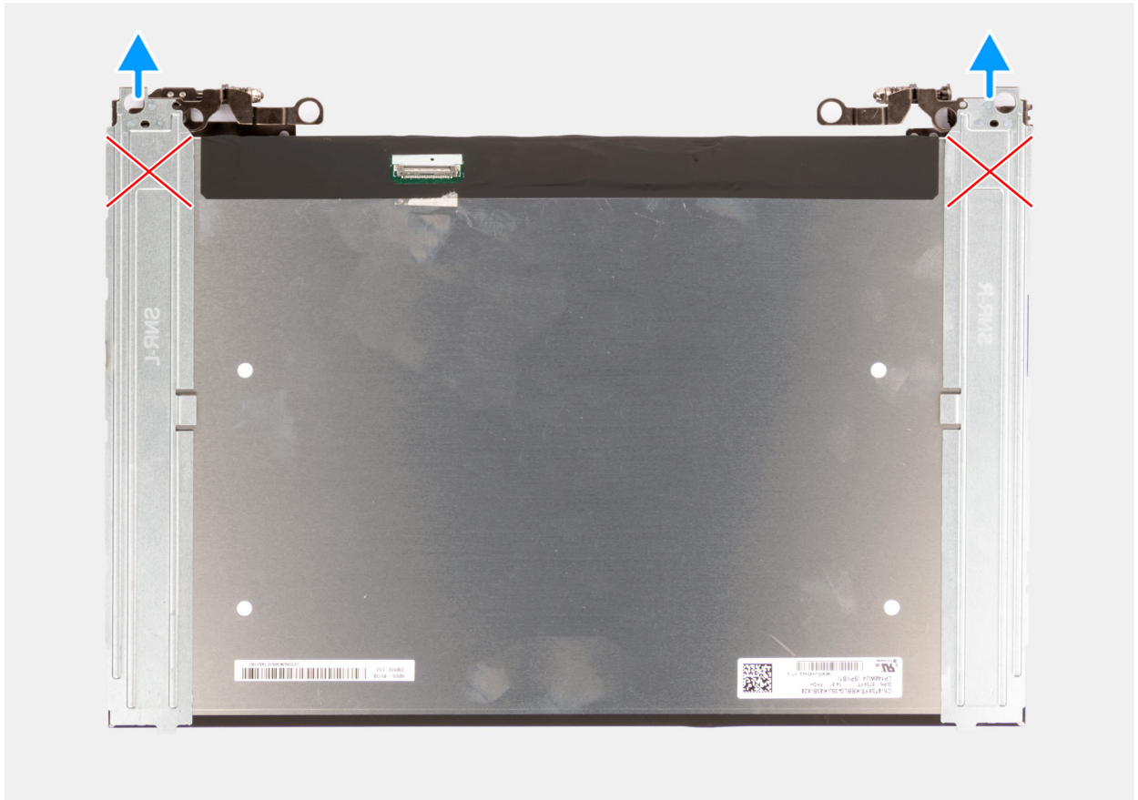
Figure 57. Removing the display panel
