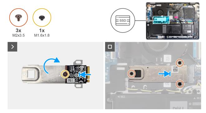
Figure 21. Installing the solid-state drive
