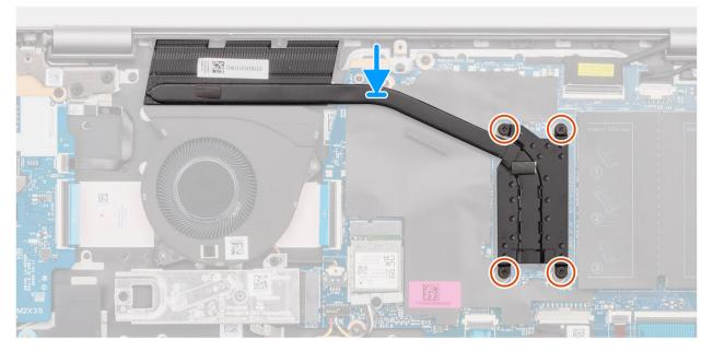
Figure 33. Installing the heat sink
