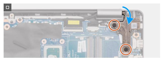
Figure 51. Installing the system board
