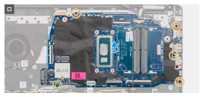
Figure 49. Removing the system board
