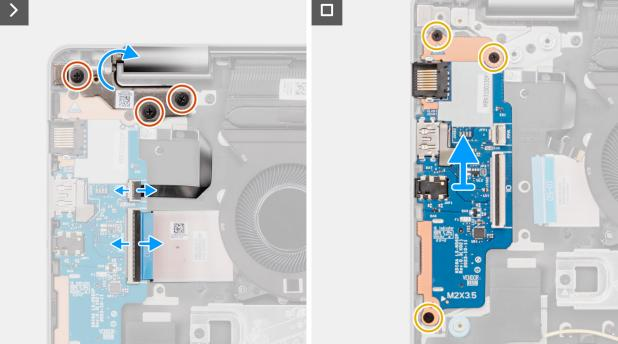
Figure 40. Removing the I/O board
