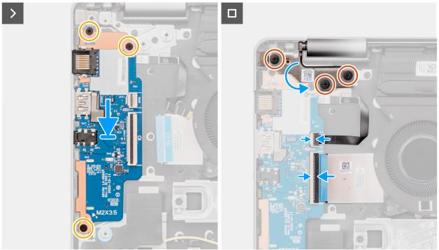
Figure 41. Installing the I/O board
