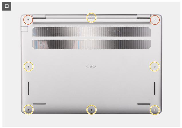
Figure 17. Installing the base cover
