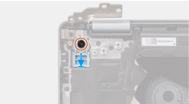
Figure 43. Installing the power button
