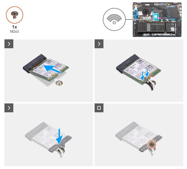
Figure 23. Installing the wireless card
