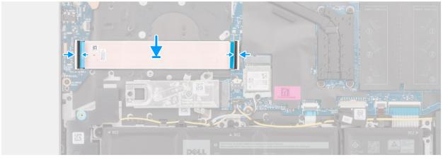
Figure 39. Installing the I/O-board cable
