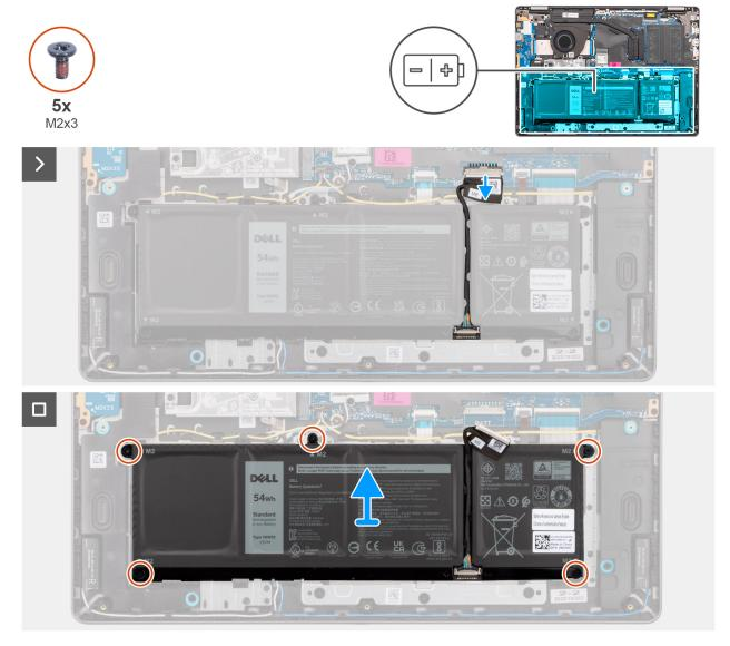
Figure 28. Removing the battery
