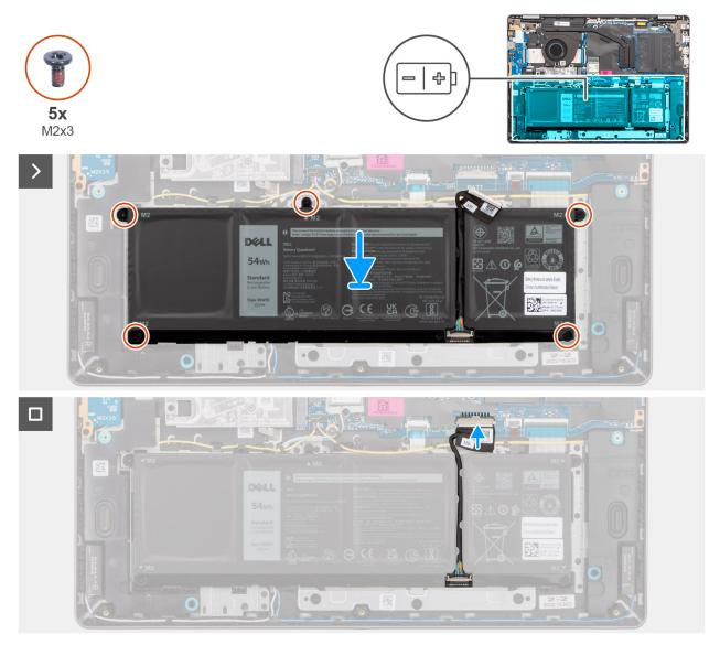
Figure 31. Installing the battery
