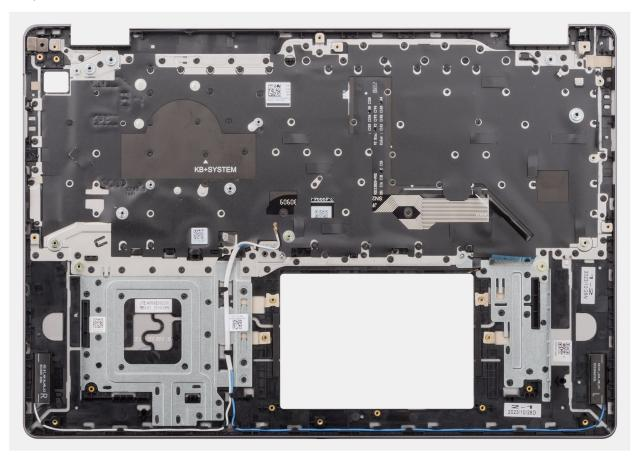
Figure 53. Installing the palm-rest and keyboard assembly
