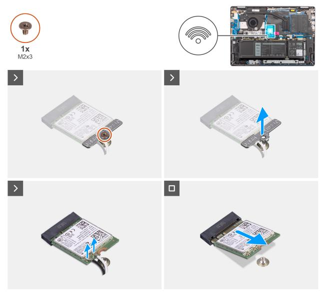
Figure 22. Removing the wireless card
