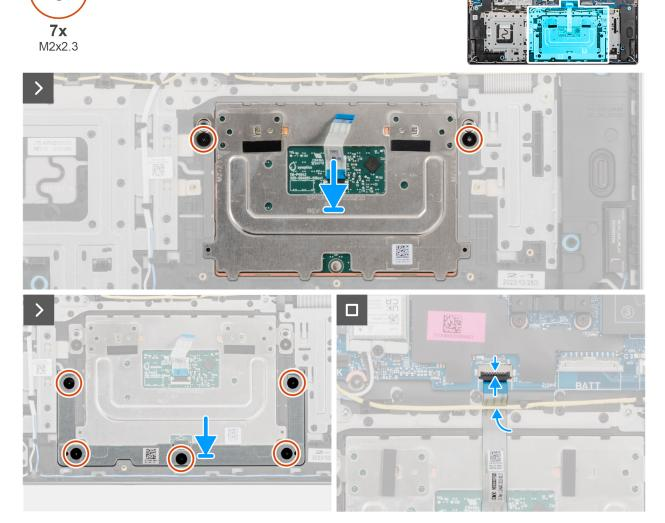
Figure 35. Installing the touchpad assembly
