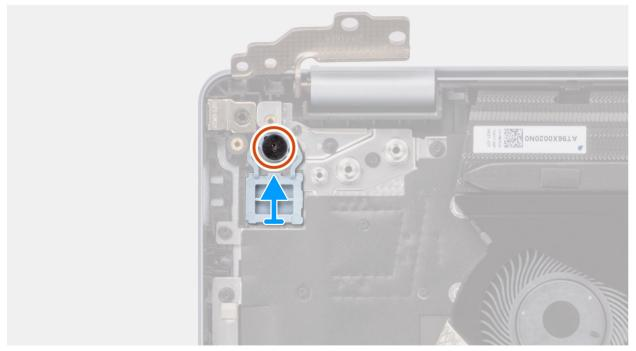
Figure 42. Removing the power button
