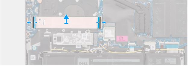
Figure 38. Removing the I/O-board cable
