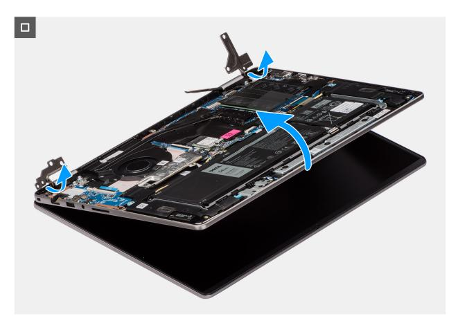
Figure 36. Removing the display assembly
