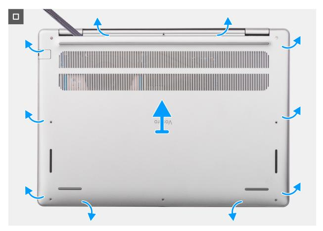
Figure 16. Removing the base cover
