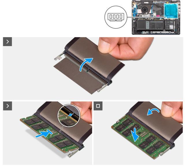
Figure 19. Installing the memory module
