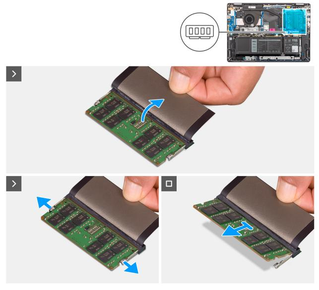
Figure 18. Removing the memory module
