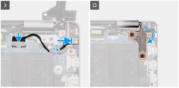
Figure 47. Installing the power-adapter port
