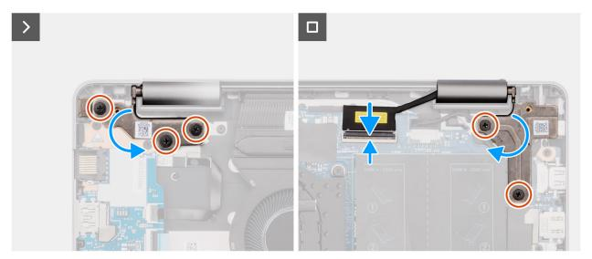
Figure 37. Installing the display assembly
