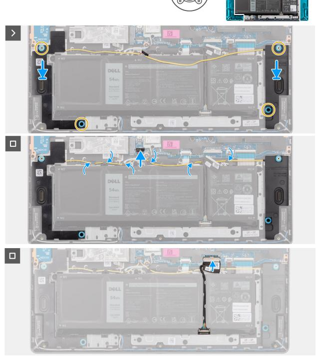
Figure 25. Installing the speakers
