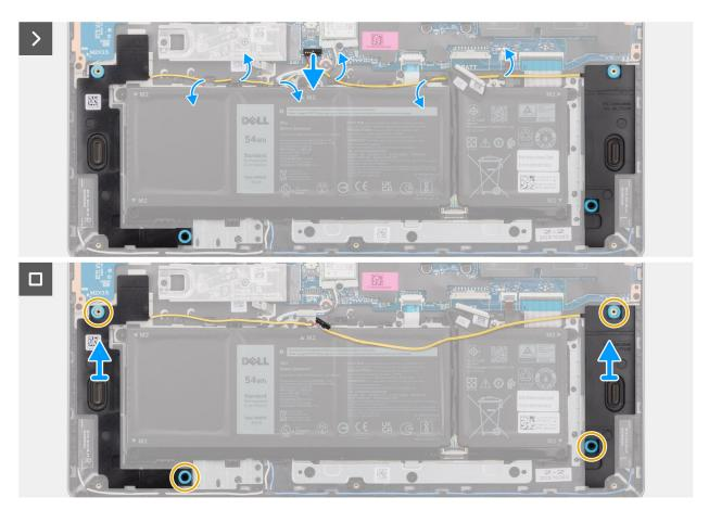
Figure 24. Removing the speakers
