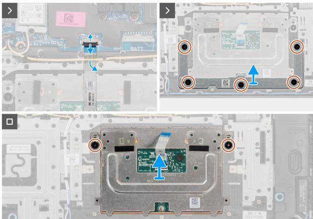
Figure 34. Removing the touchpad assembly
