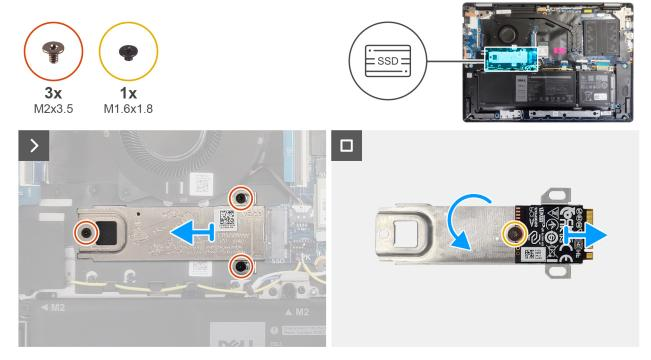
Figure 20. Removing the solid-state drive
