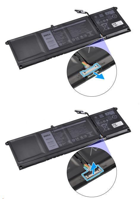
CAUTION: DO NOT pull the battery cable to disconnect it from the battery. This may damage the battery or the battery cable.
