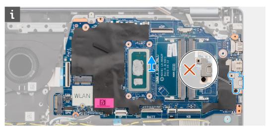
6. Carefully lift and remove the system board from the palm-rest and keyboard assembly.
