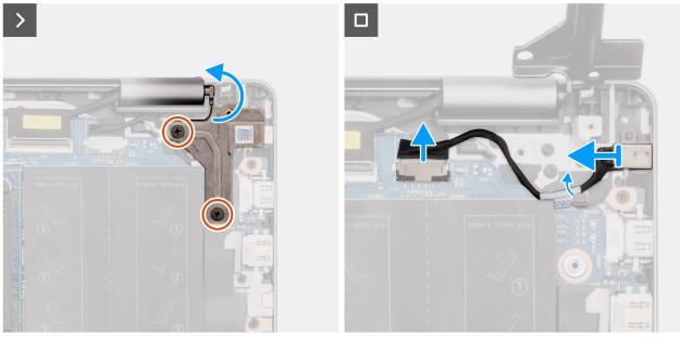
Figure 46. Removing the power-adapter port
