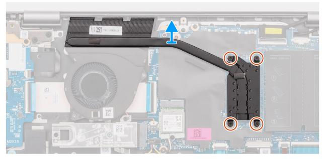
Figure 32. Removing the heat sink
