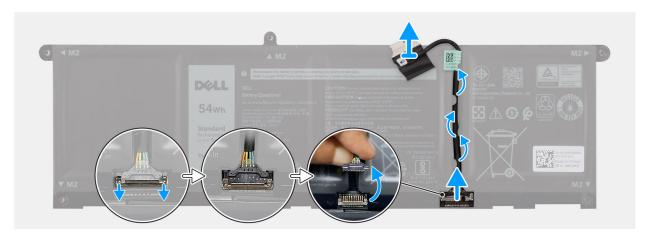
Figure 29. Disconnecting the battery cable
