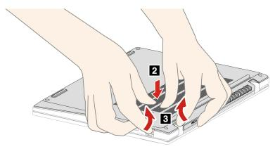
**Note:** Press the base cover assembly **2** with a pressure of less than 5 kg (11.02 lb). Release the pressure immediately when the base cover assembly is opened.
