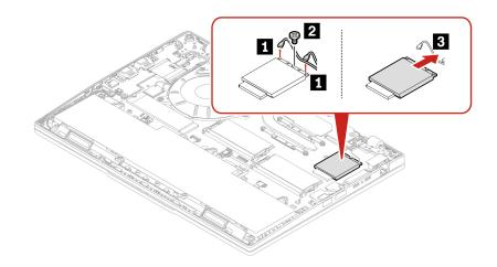
Step 2. Install the wireless WAN module as shown below.
