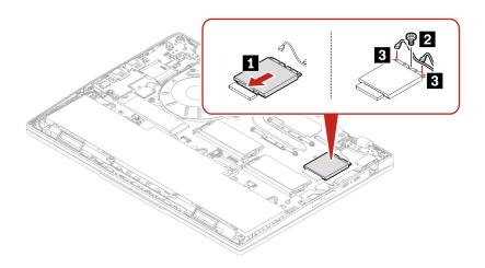
**Note:** When installing the wireless WAN module, ensure that you connect the orange cable to the connector labeled Orange on the module, and the blue cable to the connector labeled Blue.
