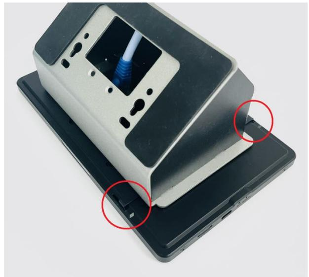
**7** Secure the Touch Panel to the mounting plate with the screw you removed at step 2.
