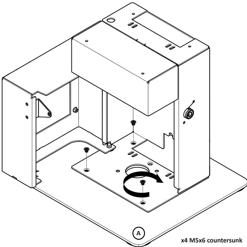
**B1** Remove back plate and place on Base plate
