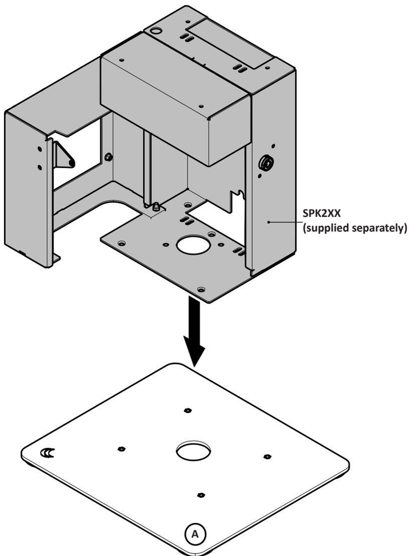
**A2** Secure Center module to the Base plate
