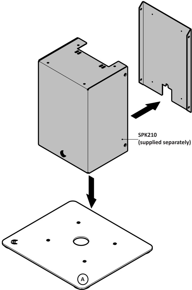
**B2** Secure Center module (blank) to the Base Plate
