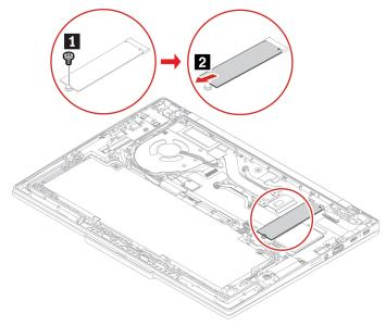
Step 2. Install the M.2 solid-state drive in reverse order.
