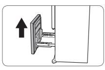
3. Lift the freezer door from the rails to remove.
