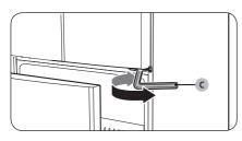
3. Turn the Allen wrench (C) clockwise or counterclockwise to raise or lower the door.
