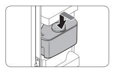
3. Reinsert the water tank and close the door. Make sure the water outlet of the water tank faces forward.
