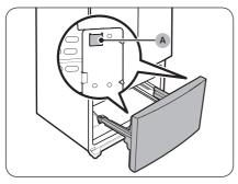
2. Attach the freezer door to the slots (A) at the side of the rails.
