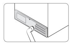
To keep cords and exposed parts of the rear panel free of dirt, vacuum the panel once or twice a year.
