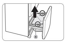
**1.** Fully open the freezer drawer, and then lift the drawer basket (A) to remove.
