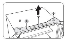
**1.** Use a Phillips screwdriver to remove the screws fastening the top cover (A).
