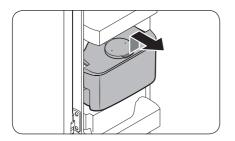
1. Hold the handgrips on both sides of the water tank and lift up to remove.
