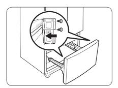
3. Use a socket wrench (10 mm) to fasten the door to the rail with 4 screws.
