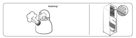
• As the refrigerator temperature increases or decreases, plastic parts contract and expand, creating knocking noises. These noises occur during the defrosting cycle or when electronic parts are working.
