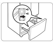
2. Use a socket wrench (10 mm) to remove the 4 screws fastening the door.
