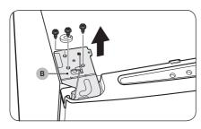
3. Use a socket wrench (10 mm) to remove the screws fastening the top hinge (B).
