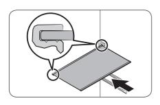
Before you insert the shelf, check the shape of the back of the shelf. Then, insert the shelf in the reverse order of removal.
