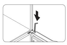
**4.** Locate the hinge shaft. While holding the door with one hand, use a flat-head screwdriver or Allen wrench to press the shaft down. Make sure to hold the door to prevent the door from falling.
