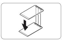
**4.** If you need to further raise the rear height, attach another adjustment pad on top of the first level adjustment pad.
