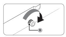
**2.** After adjusting the gap, turn the **locking** nut (B) to lock the adjustment dial.
