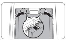
2. With the left Showcase door open, open the fridge door. Then, push the upper part of the Beverage Zone (left and right side of the fan) from inside to release the snap joints securing the Beverage Zone cover to the door.
