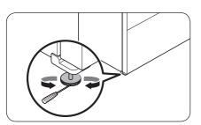
Insert a flat-head screwdriver into the leveler of the front left or right leg. Turn the leveler clockwise to raise or turn it counterclockwise to lower.
