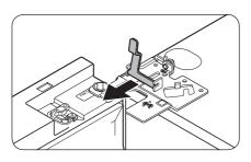
**2.** Disconnect the two wire connectors on the left door. The position of the connectors differs with the model.
