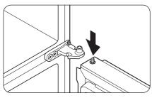
2. While pressing the hinge shaft down, position the door so that the hinge shaft is below the shaft hole in the middle hinge. Release the hinge shaft so that it enters the shaft hole.
