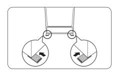
If you need to raise the rear side of the refrigerator to level it, you can use the provided level adjustment pad(s). Follow these instructions to raise the rear side of the refrigerator.
