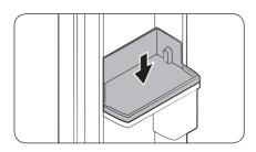
1. With the fridge door or the Showcase door open, align the grooves on the left and right side of the bottom door bin, and then insert it
