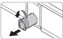
3. Turn the knob of the filter cartridge counter clockwise 90 degrees (1/4 turn). The filter cartridge unlocks.
