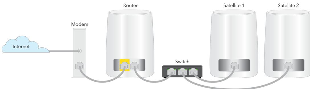
Figure 5. Ethernet backhaul connection using a switch
