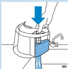
**4** Refill the water tank and reattach it to the steam generator.
