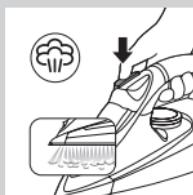
A steam boost from the special Steam Tip soleplate helps remove stubborn creases. The steam boost enhances the distribution of steam into every part of your garment. The steam boost function can only be used at temperature settings between ●●● and MAX.
