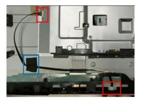
**S12** Tear off 2 conductive tapes from "Main Shielding and "Panel"
