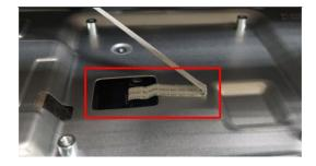
**S6** Unlock 3 screws to disassemble "Control board" from "Rear Cover"
