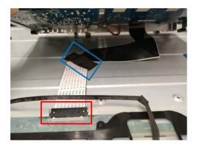
**S14** Unlock 15 screws to disassemble "Middle Frame" from "Panel"
