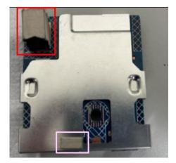
**S10** Disassemble "USB board" from "USB Shielding"
