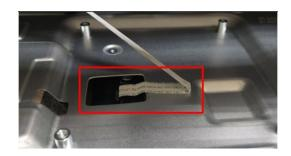
Unlock 3 screws to disassemble "Control board" from "Rear Cover"
