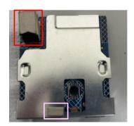
S12 Assemble "USB board" with "Middle Frame"
