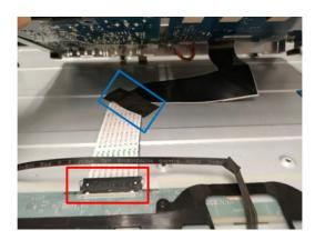
S14 Unlock 15 screws to disassemble "Middle Frame" from "Panel"
