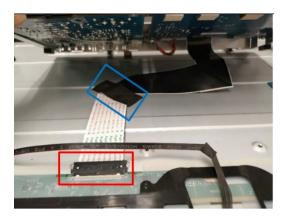
Attach 2 conductive tapes on "Main Shielding and "Panel"
