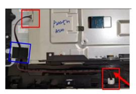
S13 Tear off 3 conductive tapes from "Main Shielding and "Panel"
