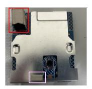
S11 Disassemble "USB board" from "USB Shielding"
