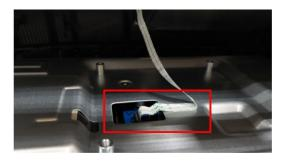
Unlock 3 screws to disassemble "Control board" from "Rear Cover"
