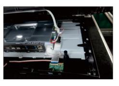
Put the rear cover into a fixture jip, then release the key cable by tearing off the tapes. Use a Philipshead screwdriver to remove 1pcs screws for unlocking the joystick key board with the rear cover.
