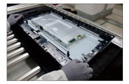
Take 1pcs panel lamp cable to connect the panel and interface board, then locate the panel lamp cable to the hook of the middle frame and fix the lamp cable on the back of panel by the tapes on the back of the cable.
