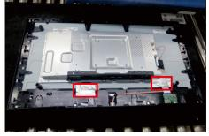
Take 1pcs joystick key, 1pcs joystick board and 1pcs joystick cable, then assemble the joystick key with board, and then connect the cable to the connector of the joystick board.
