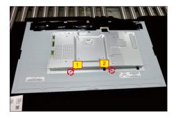
Take 1pcs middle frame to assemble the panel module, then adjust the middle bezel for two parts firmly attachment.
