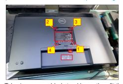
Take 1pcs assembled stand base, then fit the two tabs on the upper part of the stand into the grooves S18 on the back of the monitor, and then press the stand so that the monitor mounting area snaps onto the stand.
