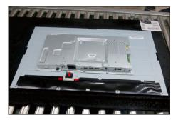
Use a Philips-head screwdriver to tighten 2pcs screws for locking the bracket with panel module.
