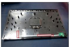
Move the assembled rear cover close to the panel, then connect the joystick cable to the connector of S16 interface board. Put down the rear cover and push the rear cover on the positions marked as the picture below shown for mechanisms engagement.
