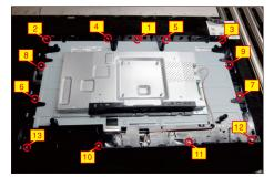
Release the IO cover from the hooks of the main bracket chassis and put it aside.
