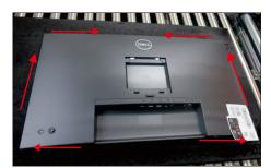
Use a Philips-head screwdriver to tighten 4pcs screws for locking rear cover with the assembled \$17 unit. Paste 2pcs labels and insert 1pcs DP cap on the specific positions as the picture below shown. (No.1~4 screw size=M4x10; Torque=10±1kgfxcm)
