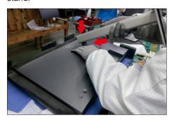
Lift up the monitor, then provide power supply and a S19 video signal to the monitor, then turn on the monitor for functionality check.
