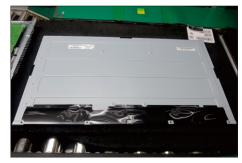
Put the bracket chassis module on the back of LCD module, then push the earing-locks and connect LVDS cable and panel lamp cable to the connectors of the panel module.
