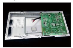
Take a interface board, connect a LVDS cable to the connector of the interface board, then connect the cable of the power board to the connector of the interface board. Turn over the interface board and locate it into the bracket. Use a Philips-head screwdriver to tighten 7pcs screws for locking the power board and interface board.
