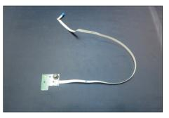
Tear off 2pcs aluminum foil, then use a Philips-head screwdriver to remove 1pcs screw for unlocking the USB unit, then disconnect the USB cable away from the board and release the USB board unit. (No.1 screw size=M3x6, Torque= $4\pm 1$ kgfxcm)
