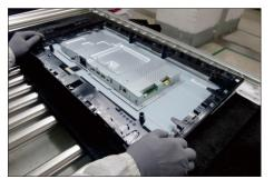
Use a Philips-head screwdriver to remove 2pcs screws for unlocking the bracket chassis with the panel.
