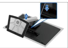
Use a Philips-head screwdriver to remove four screws for unlocking mechanisms. (No.1~4 screw size=M4x10; Torque=10±1kgfxcm)
