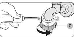
**2.** Use a Phillips screwdriver to loosen four screws on the adaptor.
