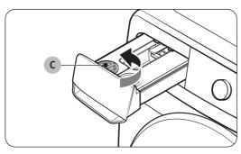
4. Turn the dispenser 2 cap (C) anticlockwise to open.
