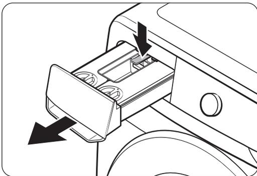
1. While holding down the **release lever** on the inner of the drawer, pull the detergent drawer to remove.
