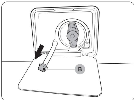
3. Place an empty, spacious container around the cover, and stretch the emergency drain tube to the container while holding the **tube cap (B)**.
