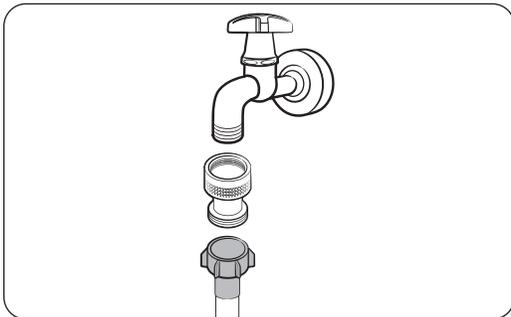
Before connecting the water hose to a water tap, connect the supplied check valve to the water tap and then connect the water hose.
