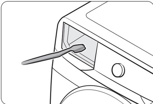
3. Clean the drawer recess using a bottle brush to remove detergent residues and limescale on the drawer recess.
