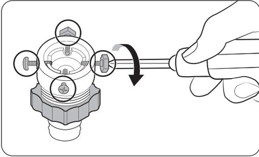
2. Use a Phillips screwdriver to loosen four screws on the adaptor.
