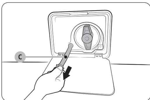
4. Open the tube cap and let water in the **emergency drain tube (C)** flow into the container.
