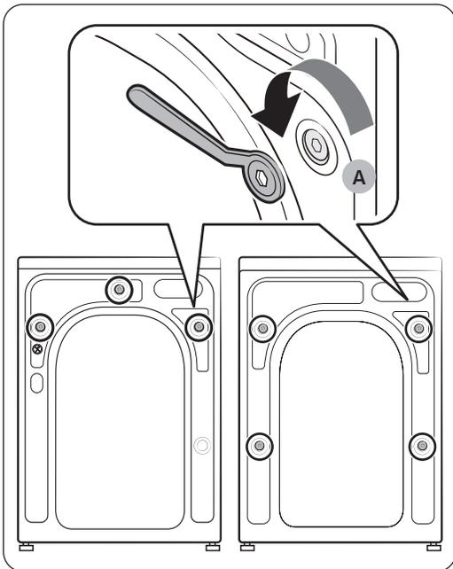
1. Locate the shipping bolts (marked with circle in the figure) on the rear side of the washing machine.
