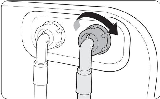
1. Connect the red end of the hot water hose to the hot water inlet on the back of the machine.
