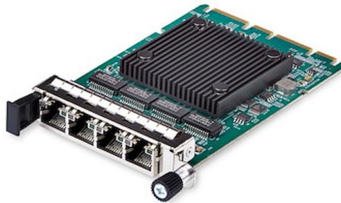
This 4-port RJ45 1Gbps OCP 3.0 Network Interface Card (NIC) features an Intel i350-AM4 Ethernet Controller, enhancing performance and data integrity. The Ethernet card adheres to OCP 3.0 standards and ensures broad compatibility, making it an ideal solution for reliable network connectivity and robust data transfer capabilities.
