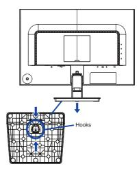
③ Press the Hook on the back of the monitor and remove the Stand-Neck from the monitor.
