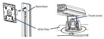
② Install the Stand-Base to the Stand-Neck and then tighten the 'thumb screw' with the provided screwdriver to secure them.
