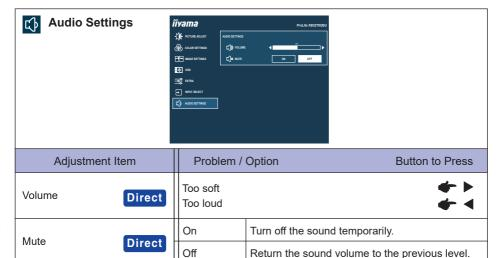
NOTE Press the ☐ Button to display the volume adjustment bar and switch On and Off the Mute function by pressing the ◀ / ▶ Buttons.
