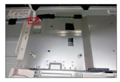
Use a Philips-head screwdriver to remove 2pcs screws for unlocking the joystick key board unit, then S7 tear off the tapes and release the USB board.
