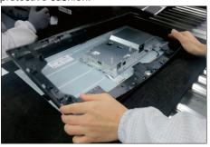
Move up the bracket chassis module, and
