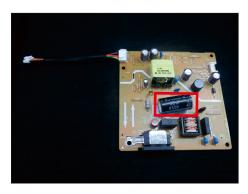
S17-1 Cut the glue between bulk cap. and PCB with a knife.
