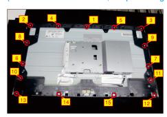
Use a Philips-head screwdriver to remove 1pcs screws for unlocking the IO cover, then release the IO cover from the hooks of the bracket chassis.
