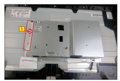
S11 Tear off 3pcs aluminum foil for releasing the bracket chassis module.
