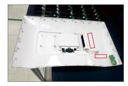
Use a Philips-head screwdriver to remove 1pcs screw for unlocking the IO cover, then release the IO cover from the hooks of the bracket. Tear off 4pcs acetate tapes to release speakers' cables.
