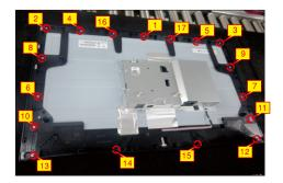
S11 Tear off 3pcs aluminum foil for releasing the bracket chassis module.
