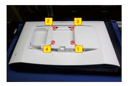
Use a mylar sheet to insert the left-bottom corner to release the rear cover, then wedge your fingers between the rear cover and the middle bezel of the monitor to release the rear cover, then use one hand to press the middle bezel, the other hand to pull up carefully the rear cover in order of arrow preference for unlocking mechanisms of rear cover.
