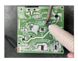
S17-5 Lift the bulk cap. up and away from the PCB.
