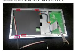
Use a Philips-head screwdriver to remove 6pcs screws for unlocking the circuit board.
