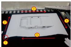
S6 Lift the rear cover up carefully. Disconnect the joystick cable from the connectors of the interface board, and then remove the rear cover and put it aside for later disassembling.
