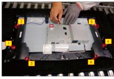
Use a Philips-head screwdriver to remove 15pcs screws for unlocking the middle frame with the panel module.
