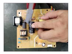
S17-3 Cut into the bottom of bulk cap. and pullit up carefully.
