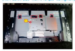
Use a Philips-head screwdriver to remove 6pcs screws for unlocking the speakers, then disconnect the speakers' cable away from the connector and release the two speakers from the hooks of the middle frame.
