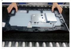
Move up the bracket chassis module, and disconnect the LVDS cable and panel lamp cables from the connectors of the panel, then tear off the tapes and lift up the bracket chassis and put it aside for later disassembling.
