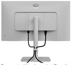
Remove stand from the product.(Press the stand release button, lift the stand up and away from the monitor)
