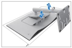
Use a Philips-head screwdriver to remove 4pcs screws for unlocking rear cover with assembled unit.
