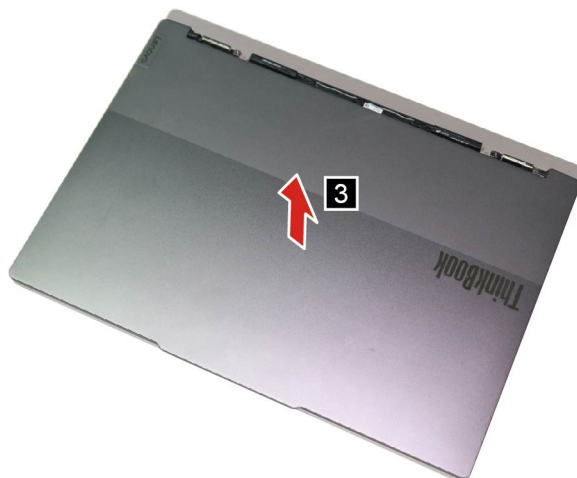
Figure 45. Remove the LCD module
