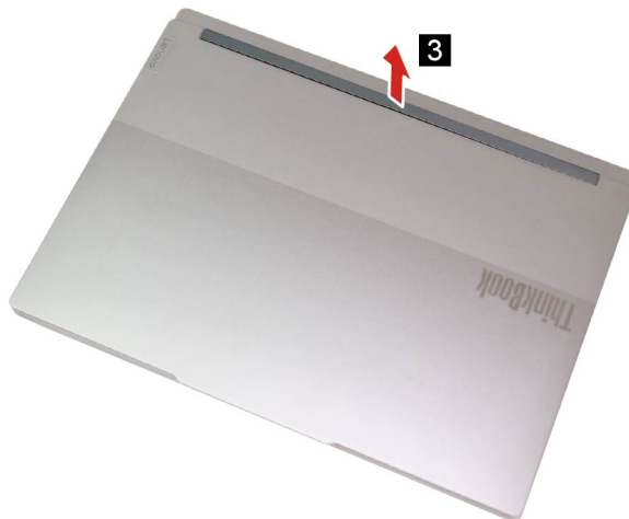
Figure 43. Remove the hinge cap
