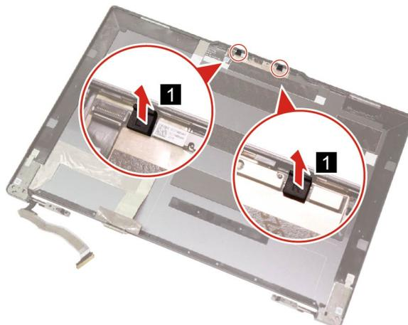
Figure 52. Remove the microphone rubbers
