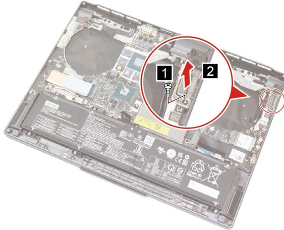
Figure 36. Remove one screw and the USB-A bracket
