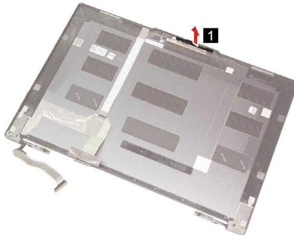
Figure 51. Remove the camera shutter
