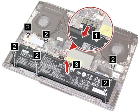
Figure 6. Remove six screws and the battery pack
