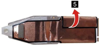
Figure 14. Peel off the SSD Cu foil mylar
