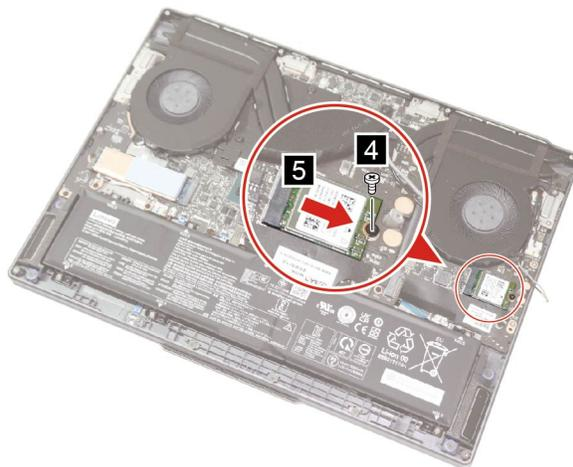
Figure 24. Remove one screw and the Wi-Fi card
