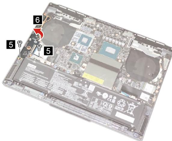
Figure 35. Remove two screws and the I/O board
