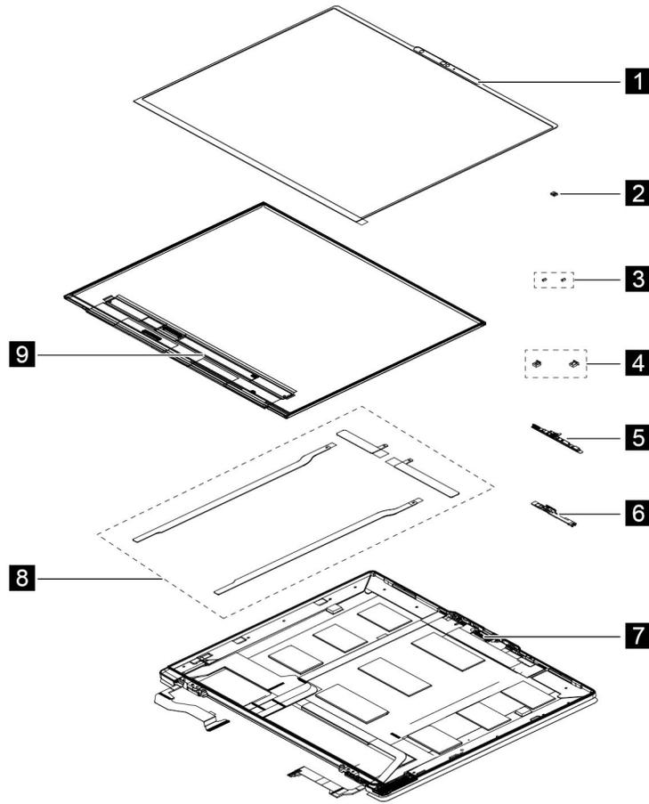
Figure 2. LCD exploded view
