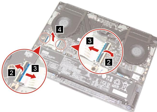
Figure 32. Disconnect and remove the I/O board cable
