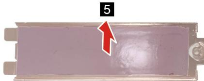
*Figure 11. Remove the 2280 SSD thermal pad*
