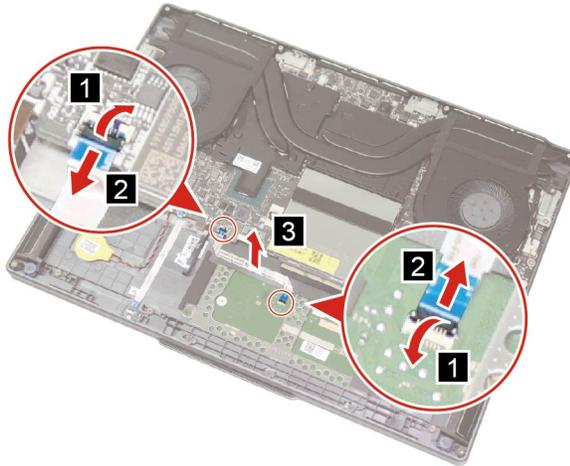
Figure 16. Disconnect and remove the touchpad cable
