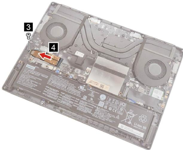
Figure 13. Remove one screw and the 2242 SSD module
