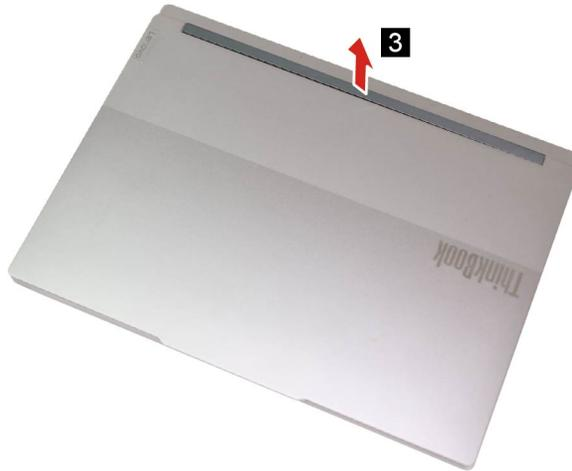
Figure 43. Remove the hinge cap
