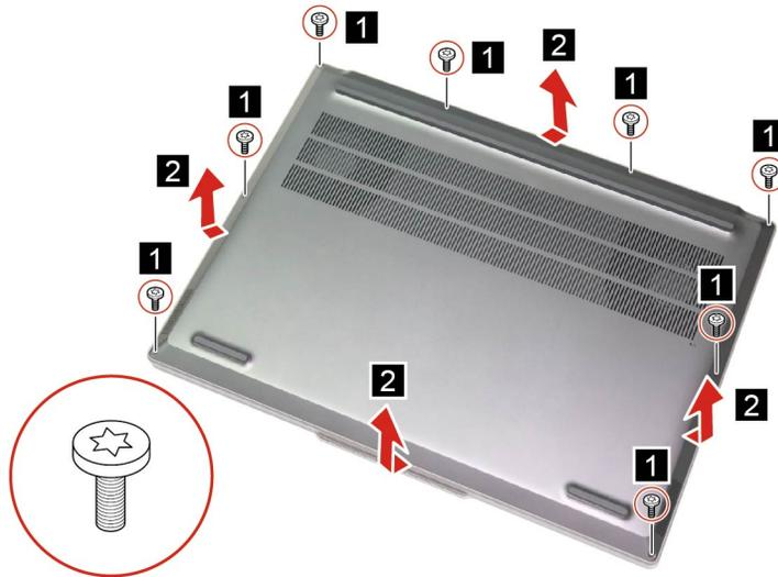
Figure 5. Remove eight screws and the lower case
