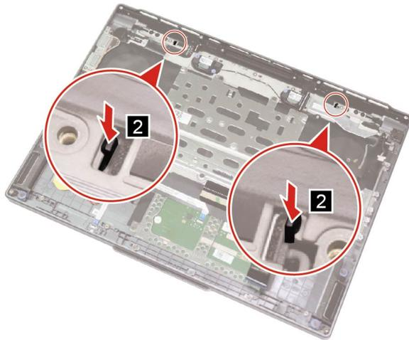
Figure 42. Release the hooks
