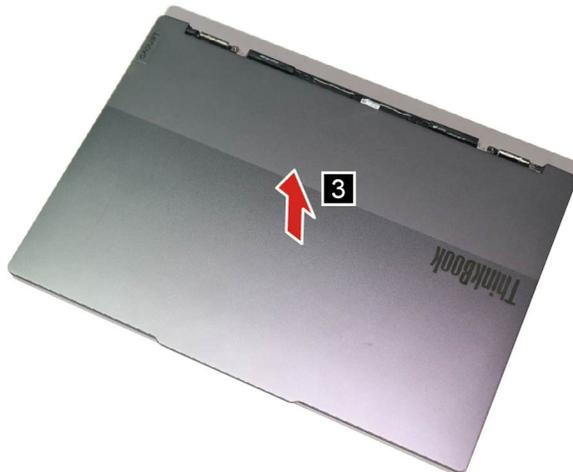
Figure 45. Remove the LCD module
