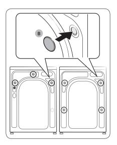
**3.** Insert the **bolt caps (B)** to the holes (marked with circle in the figure).
