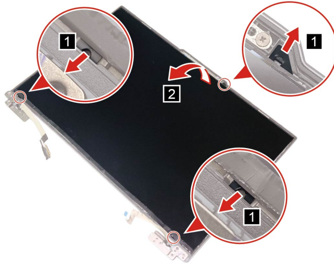
Figure 33. Pull out three adhesive tapes
